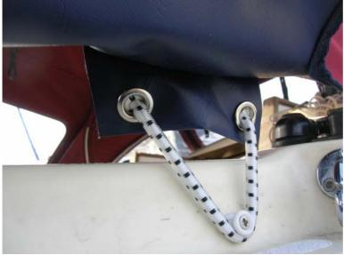
Typical cover attachment bungee & lacing stud on cockpit coaming
